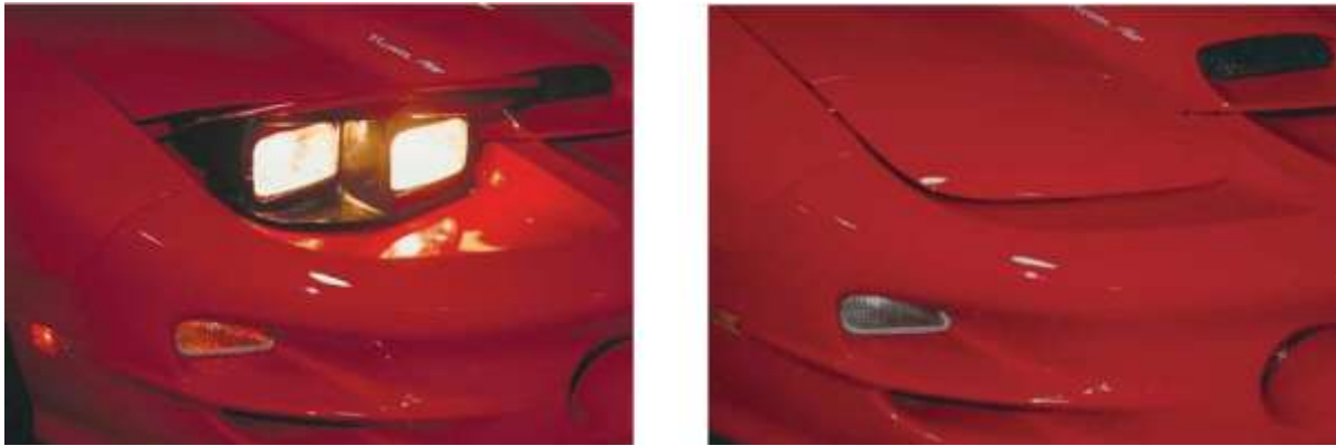
FIGURE 2-17 Concealed headlights enhance the vehicle's styling and aerodynamics.
