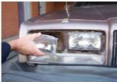
P15-4 Remove the headlight from the shell assembly.
