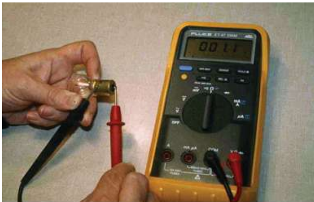
FIGURE 2–36 often the best diagnosis is a thorough visual inspection. This bulb was found to be filled with water, which caused weird problems.
