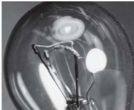
Figure 2–34 Close-up a 2057 dual-filament (double contact)bulb that failed. Notice that the top filament broke from its mounting and melted onto the lower filament. This bulb caused the dash lights to come on whenever the brakes were applied.
