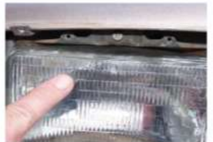
P15-9 Place the headlight into the shell assembly. When positioning the headlight, be sure that the embossed number is at the top. Many headlights are marked "TOP."
