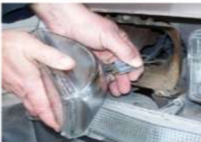
P15-8 Install the wire connector onto the new headlight's connector prongs.
