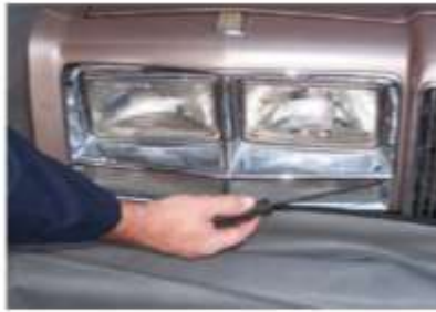
P15-2 Sealed-beam headlight replacement usually requires the removal of the bezel. Some vehicles may require that the turn signal light assembly be removed before the headlight is accessible.
