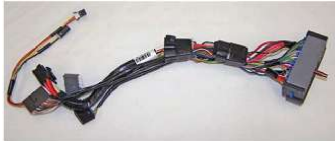
Figure 2- 1 typical partial wiring harness that connects to a connector on the fire wall.
