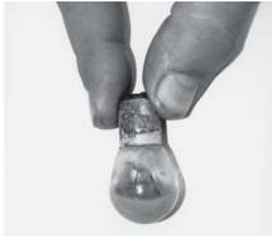
FIGURE 2–36 often the best diagnosis is a thorough visual inspection. This bulb was found to be filled with water, which caused weird problems.
