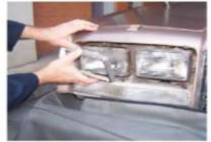
P15-3 Remove the retaining ring screws and the retaining trim. Do not turn the two headlight aiming adjustment screws.
