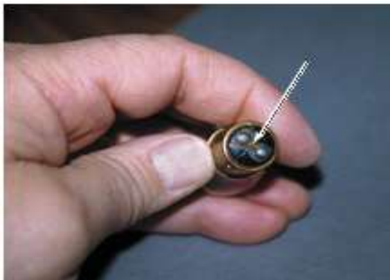
FIGURE 2–35 Corrosion caused the two terminals of this dual-filament bulb to be electrically connected.
