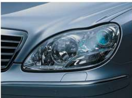
FIGURE 2-12 HID headlamps; note the reduced size of the headlamp assemblies.
