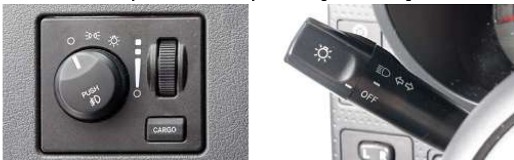
FIGURE 2-20 (A) Instrument panel-mounted headlight switch. (B) Steering column-mounted headlight switch.
