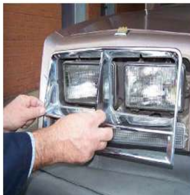
P15-11 Install the headlight bezel.
