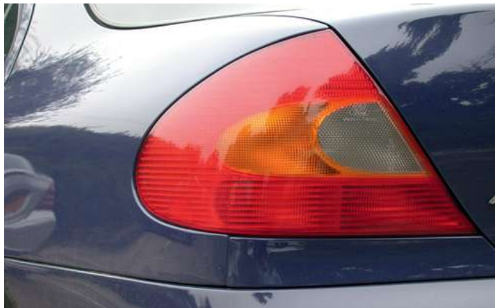
Figure 2-28 Stop and reverse lights form part of the rear light cluster
