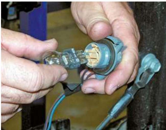
Figure 2–54 Many light bulbs are pulled out or pushed into their sockets.
