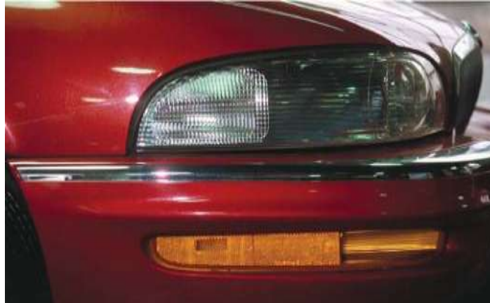
FIGURE 8-27 Cornering lights are used to provide additional illumination during turns.
