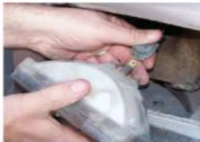
P15-5 Disconnect the wire connector from the back of the lamp.
