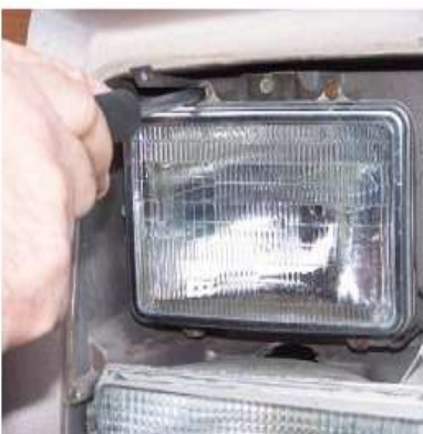
P15-10 Install the retainer trim and fasteners.
